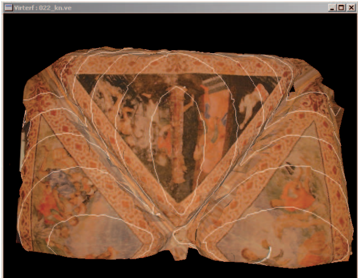
Figure 6. Model of the vaults of the "Salle Héraldique" in the Arenberg Castle in Leuven, iso-lines generated
