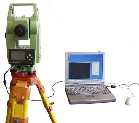
Figure 3. Total Station with real-time Visualisation
